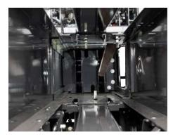
**Compression chamber** Interior of compression chamber size 34x44 cm (for M60), 36X46 CM (FOR M61) and trolley.
