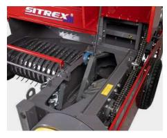
Focus on the gear reducer.
