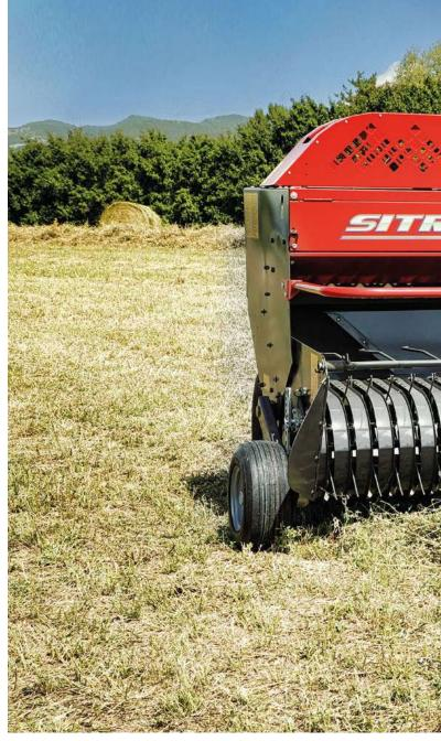
M6O and M61 are machines that can be used with low-power tractors thanks to their light weight and manoeuvrability. They are suitable for mountainous areas and steep slopes. They allow for tight manoeuvring, especially the smaller models. They have an excellent harvesting capacity and a good bale production capacity. The bales can be easily adjusted in terms of length and density, thus allowing for easy manual handling and harvesting. Both hay and straw can be baled effortlessly.
