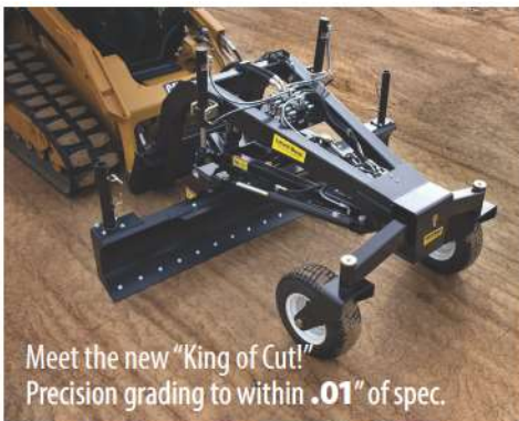
Side-shift to reach and place windrow.
