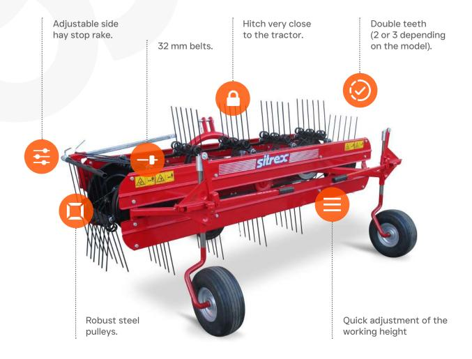
Works quickly on any green or dry forage without damaging it thanks to the perfect elasticity of the tines which adhere to any type of soil permitting an excellent cleaning during the raking and moving phases. The windrow formed by the SITREX belt rake is never a long braid but rather a soft and light windrow. Exceptional performance in turning any kind of forage even at high forward speeds. All the ball bearings are watertight and require no lubrication.
