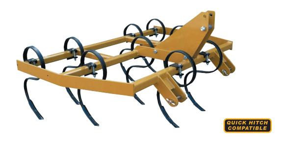
RST SERIES S-TINE CULTIVATORS are ideal for pastures, orchards, vineyards and general fieldwork. Available in 4', 5', 6', 7', 8', 10' and 12' sizes and designed for tractors 15-70 HP. The 2" square, 3-bar frames are reinforced and equipped with heavy-duty 3/8" x 1-1/4" x 16" clearance S-tines and reversible points on 6-1/2" spacing. Optional equipment includes 2-5/8" duck foot; 4" and 7" sweeps, and a pair of pin adjustable gauge wheels.
