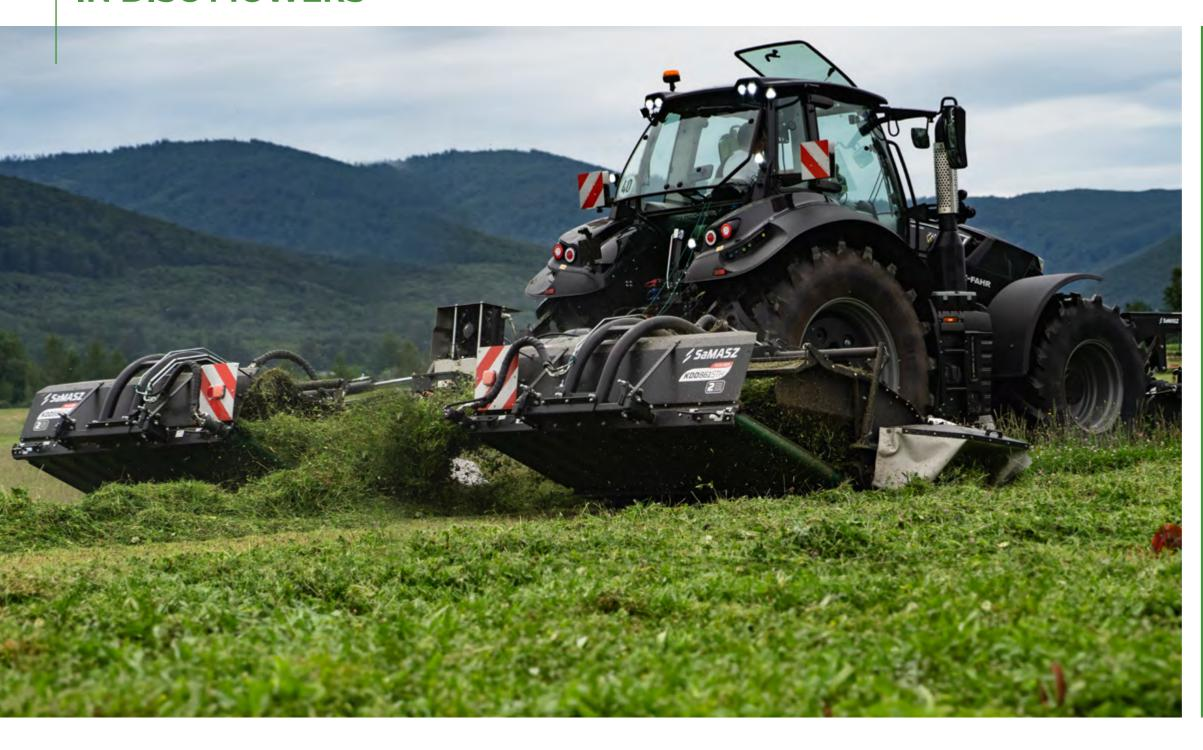
Conditioner – a tool for efficient harvesting of forage. A key element that will be appreciated by users who want to speed up the drying process of mowed material, eliminating the need for tedding. They are available in two variants: a flail conditioner and a roller conditioner, and allow to suit to individual needs of a user ensuring unique benefits when harvesting plants.
