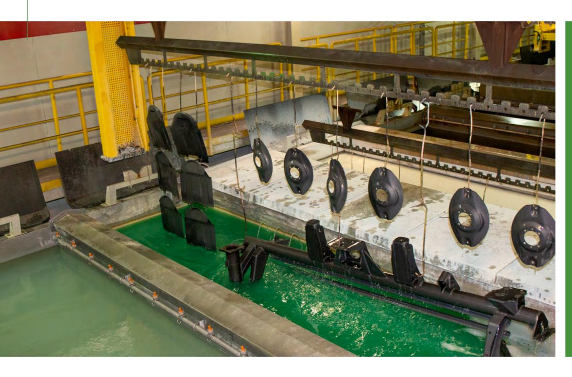
Cataphoretic painting (E-COAT) is used to cover elements that require coatings with significant corrosion resistance. At SaMASZ this process is carried out in a fully automated method. Each step is continuously monitored and archived, ensuring the repeatability of the process and the highest coating quality. In addition, it provides high weather resistance, corrosion protection, chemical and mechanical protection and an eyecatching design.
