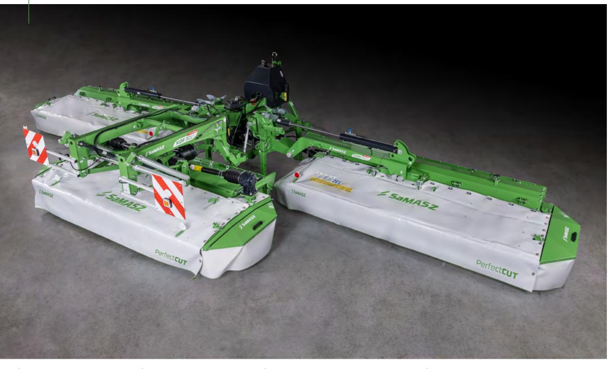
KDD-R - a combination of a front mower with KDD, a two-sided rear one on a one frame. Specially designed set for mounting with tractors with reverse system. The great advantage of the KDD-R is the ideal visibility of the entire mower combination within the operator's field of sight. It is the ideal solution for work on large farms and for service providers.
