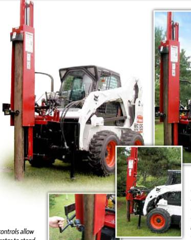
A patented safety arm attachment holds the post in position, providing added safety for the operator.
