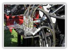
Offset controls allow the operator to stand safely to the side of the unit while posts are being driven.
