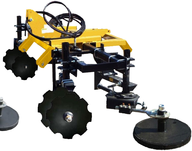
3-Point Mount shown with RH & LH Spin Weeder Assemblies, RH & LH 3-Blade Adjustable Disc Cultivators
