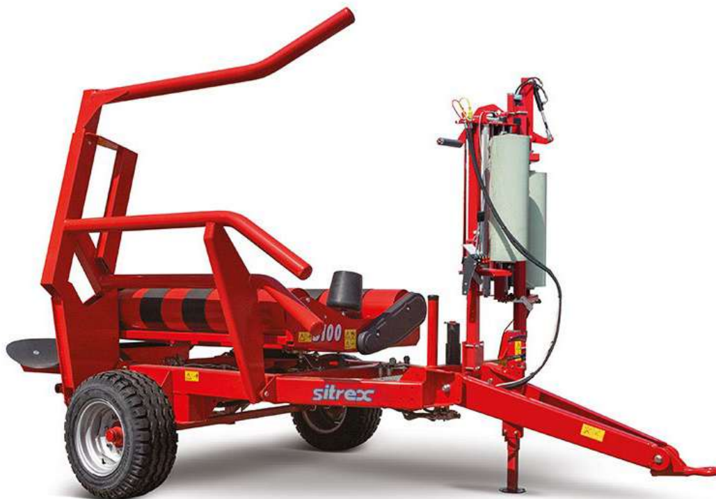
Rear platform to unload bale or vertical overturning
